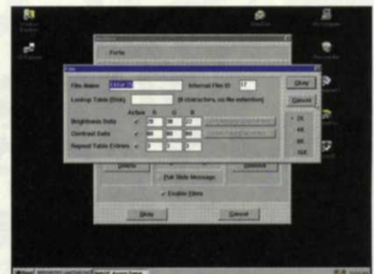
Modification of LUTs in film recorder driver software
